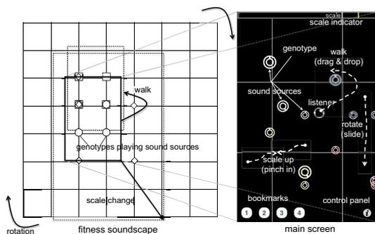
**Fig. 2.** Basic operation of the iSoundScape App (left) and a snapshot (right) of the main screen, with labels described in the text
